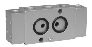
Pneumatically actuated 5/2-way spool valve with actuation by impulse. If pressure is applied to 14, the valve is open from 1 to 4 and 2 to 3, 5 is closed. If pressure is applied to 12, the valve is open from 1 to 2 and 4 to 5. Interface according to Namur standard.
