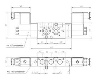
5/3-way solenoid valve with spring return to middle position, actuated by permanent signal, normally closed. Interface according to Namur standard.
