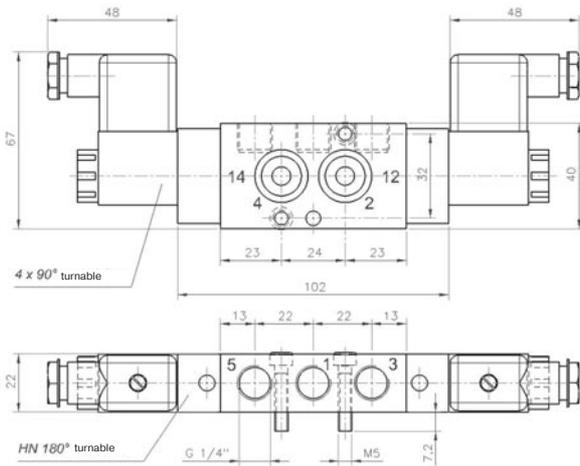
5/2-way solenoid valve actuated by impulse. Position is kept until next electrical sign even when not attached to electrical source. Interface according to Namur standard.
