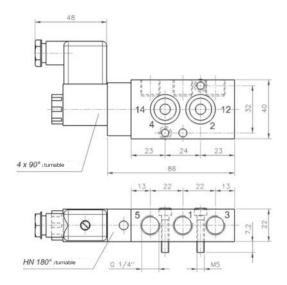
The valves are generally equipped with manual override to turn (standard). If requested without manual override, please order MN 510 70A.
