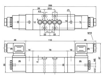
5/3-way solenoid valve with spring return to middle position, actuated by permanent signal. All ports are in the manifold plate.
