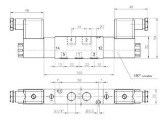
5/3-way solenoid valve with spring return to middle position, actuated by permanent signal. Ports 2 and 4 are at the valve, ports 1, 3 and 5 at the manifold plate.
