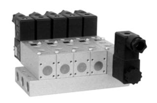
5/3-way solenoid valve with spring return to middle position, actuated by permanent signal. Ports 2 and 4 are at the valve, ports 1, 3 and 5 at the manifold plate.
