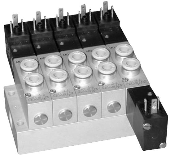
5/3-way solenoid valve with spring return to middle position, actuated by permanent signal. Ports 2 and 4 are at the valve, ports 1, 3 and 5 at the manifold plate.
