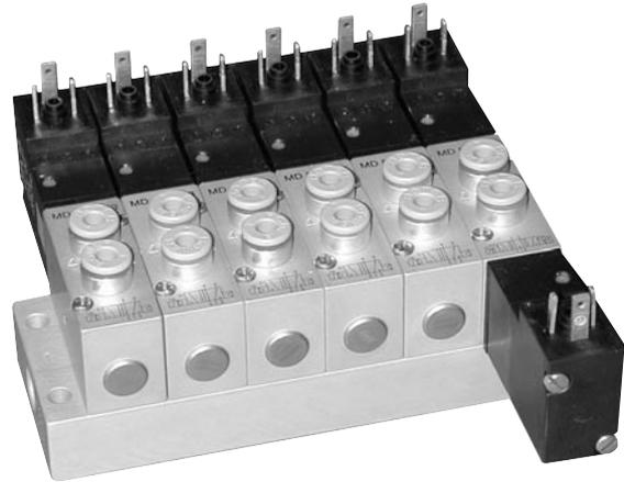
5/3-way solenoid valve with spring return to middle position, actuated by permanent signal. Ports 2 and 4 are at the valve, ports 1, 3 and 5 at the manifold plate.
