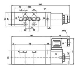
5/2-way solenoid valve with air spring, actuated by permanent signal. All ports are in the manifold plate.
