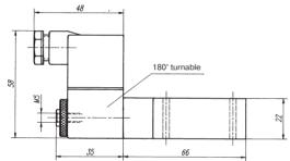
5/2-way solenoid valve with air spring, actuated by permanent signal. All ports are in the plate.
