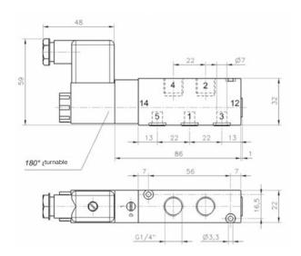
5/2-way solenoid valve with air spring, actuated by permanent signal. Ports 2 and 4 are at the valve; 1, 3 and 5 at the manifold plate.
