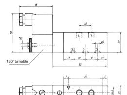
5/2-way solenoid valve with air spring, actuated by permanent signal. Ports 2 and 4 are at the valve; 1, 3 and 5 at the manifold plate.
