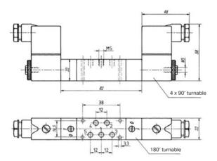
5/2-way double solenoid valve, actuated by impulse. Position is kept until an electrical signal is applied to the opposite side, even when not attached to electrical source.
