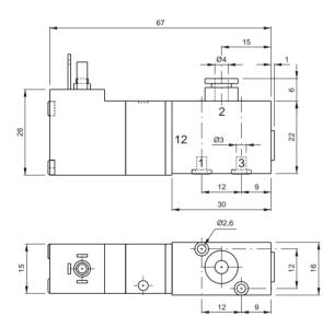
3/2-way solenoid valve, normally closed (MD) or normally open (MOD), for assembling on a manifold plate, with push-in fitting at port 2.
