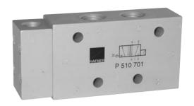
Pneumatically actuated 5/2-way spool valve with air-spring, actuated by permanent signal.
