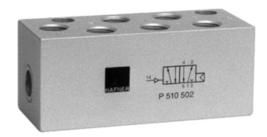
Pneumatically actuated 5/2-way spool valve with air-spring, actuated by permanent signal at 14.
